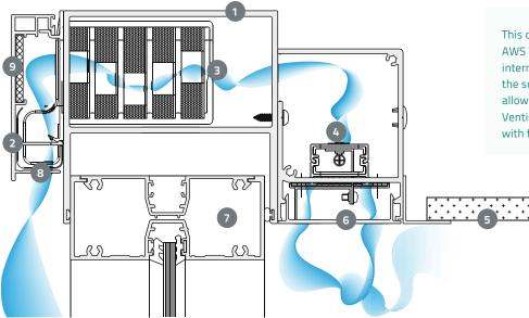
This configuration shows the AWS Ventient<sup>™</sup> housed within an internally mounted box fixed to the sub-head. This configuration allows access to the AWS Ventient<sup>™</sup> device when installed with flush plasterboard ceilings.
