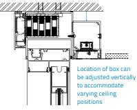
AWS has developed a number of alternate installation configurations for Ventient™ devices allowing the AWS Ventient™ to be fully integrated with AWS high performance windows and doors. Choose from one of six configuration
