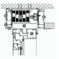
Standard configuration shows the AWS Ventient<sup>™</sup> device mounted within sub-head. Optional angle bracket to accommodate suspended ceiling tile.
