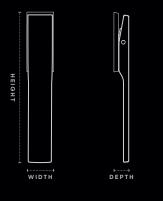
Height 149mm Width 27mm Depth 15mm
