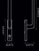
Handle 253mm Height 160mm <u>34mm</u> Width Depth 71mm
